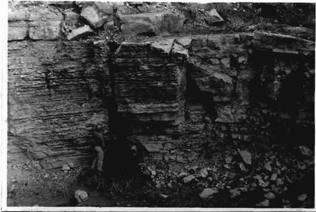
A. Lower face of quarry in the Plattin limestone showing pitting on the fucoidal phase and jointing. West side of Highway 47, NW \frac{1}{4} , Sec. 33, T. 46 N., R. 2 W.
